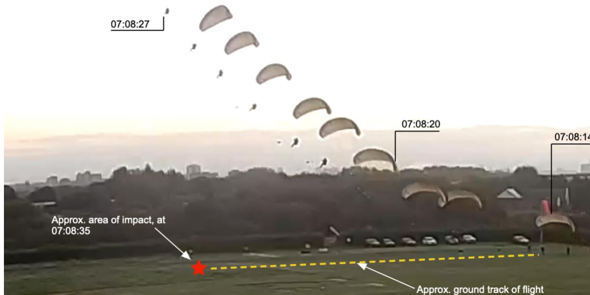
Fig. 3. Composite image of Pilot A's flight sequence captured by airfield camera, produced from stills.
