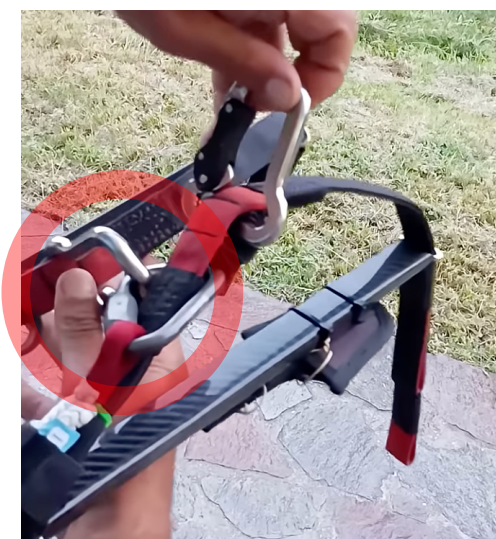
Image 2: Emergency parachute maillon now locked in the carabiner – spreaders and risers now fastened together (highlighted in red).
