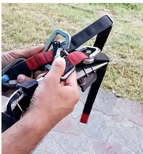
Image 1: Emergency parachute bridle maillon slides against opposite spreader carabiner button and gate, allowing it to open.
