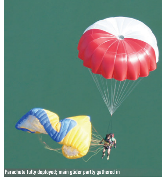
Parachute fully deployed; main glider partly gathered in
