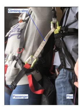
The issues come from the loads applied to the pilot harness and carabiners. The carabiner manufacturers consulted stated that their carabiners cannot be used for multidirectional loads in this way. Additionally, the webbing loop to the carabiner can foul the gate and cause wear. Whether climbing slings are used or not, the problem still exists.
