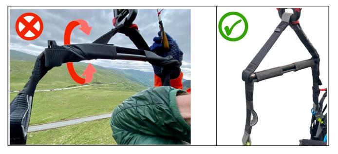
The spreaders on the photographs are "Hard Hybrid" spreaders manufactured by Advance. The majority of incident reports relate to these spreaders, but the issue is not exclusively with this specific spreader from this manufacturer.
