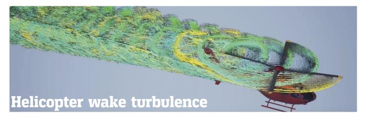
Following a fatal incident in which a coastal-flying paraglider was downed by a helicopter landing on an adjacent beach, the BEA (French equivalent of the UK's AAIB) conducted an investigation into helicopter wake turbulence. Their findings are summed up in a short video at
