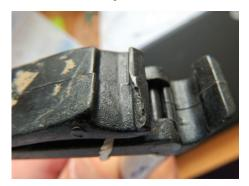
inspecting their own batten clips. Many of these used on imported gliders are to very similar designs. Some pilots have discovered hitherto-unnoticed damage (see photo at left) to these clips allowing them to open under very light loads. All hang glider pilots owning or flying gliders with these clips are encouraged to check them very carefully and replace any that are damaged. The consequences of these opening in flight are uncertain and could be very dramatic.
