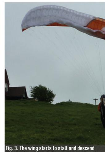
Fig. 3. The wing starts to stall and descend
