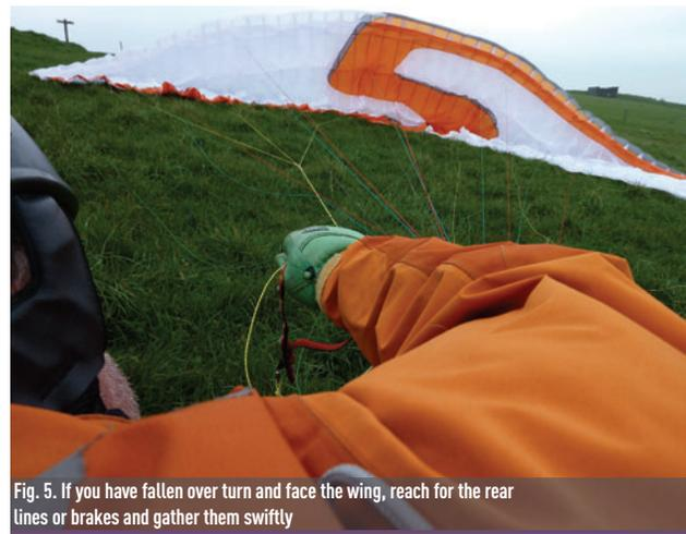
Fig. 5. If you have fallen over turn and face the wing, reach for the rear lines or brakes and gather them swiftly
