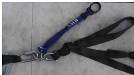
Figure 2: In this picture the D-bag is on the left, the quick release (with the blue strap) is in the middle, and the suspension points to the harness are on the right.
