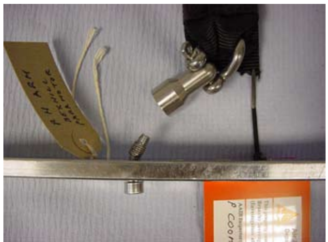
Figure 4 Right lift arm, threaded connection
